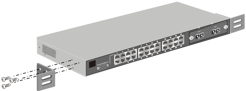
Figure 2- 2A. Attaching the mounting brackets to the switch
